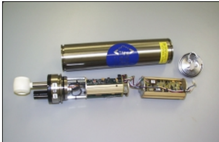
Figure 3 Complete MCTD with DPSK Module
