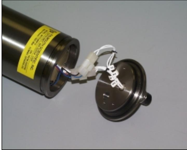
Figure 2 Inline Sea Cable and RS-232 Harness before Final End Cap Assembly
