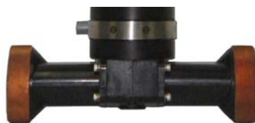
Cell Type A: Potted NXIC-BIO cell
