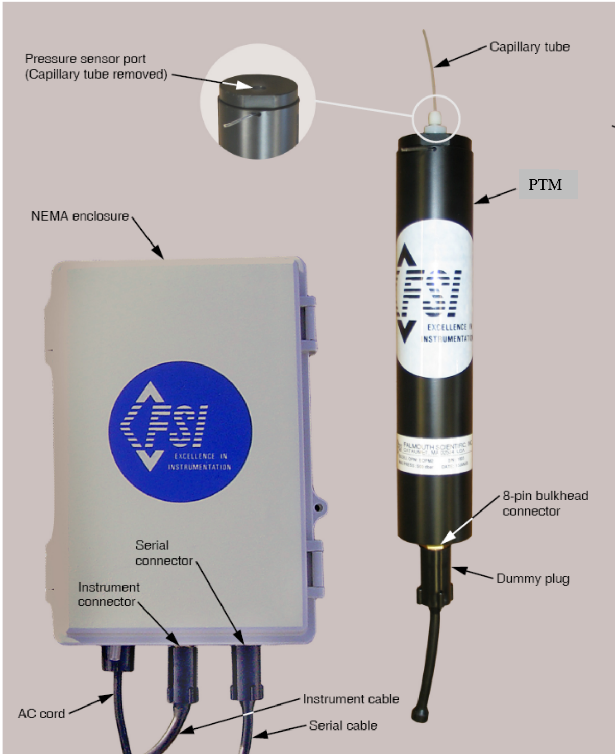
Figure 1-1: The PTM Tide System Components
