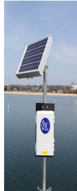
Tide System with optional solar charger
