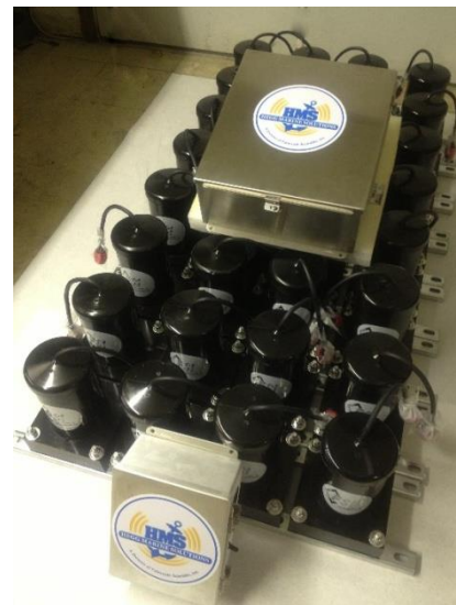
32 Element 12KM LF Array with Preamp and Junction Box
